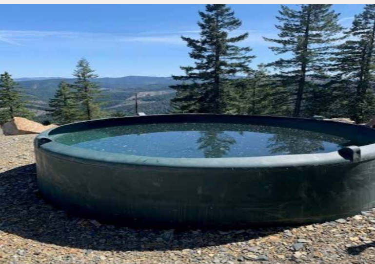
Figure 2. Water Dip Tanks are used in western United States to allow helicopters to efficiently manage fires.
